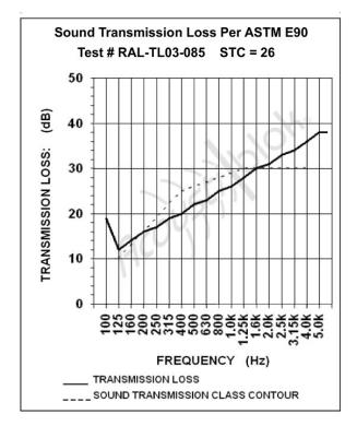
SOUND TRANSMISSION CLASS is a single number that represents the sound blocking capacity of a partition such as a wall or ceiling.
